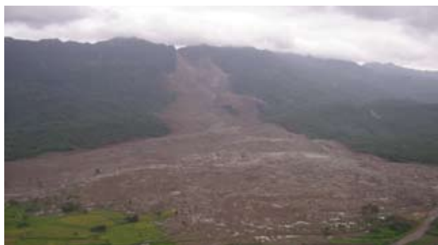
Figure 3.10 A large-scale rapid landslide triggered by a small nearby earthquake, five days after a heavy rainfall in February 2006 in the Philippines, claimed more than 1,000 lives. (Taken by Kiminori Araiba)
