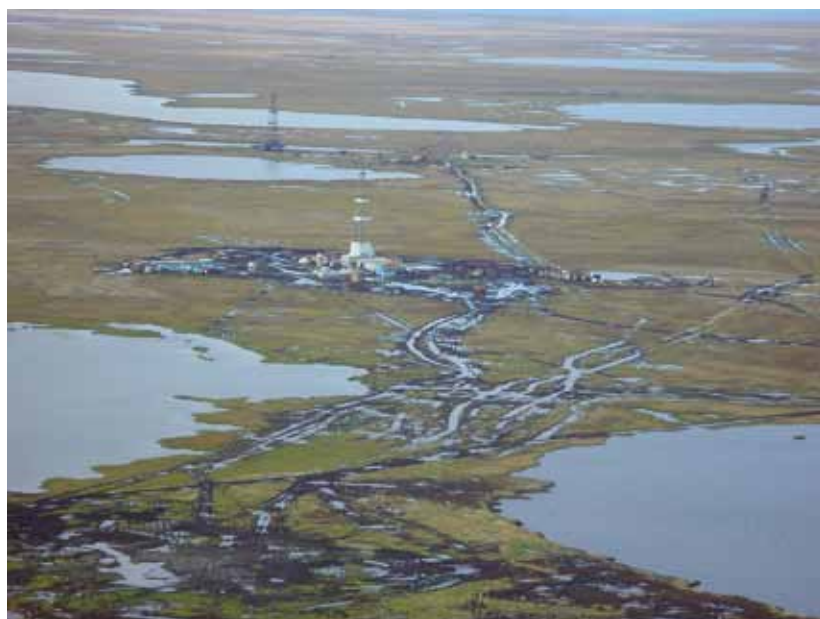
Fig. 3.10-1. Vehicle tracks across summer tundra near the oil terminal Varandey; driving on unfrozen ground leads to a rapid destruction of the tundra cover and is considered an unlawful activity in Russia, though rarely prosecuted.
