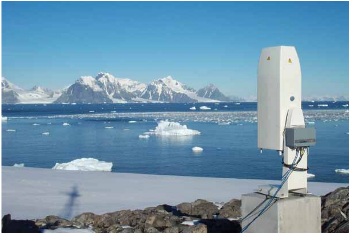
Fig. 3.5-4. Vaisala CT25K cloudbase recorder at Rothera (U.K.).
