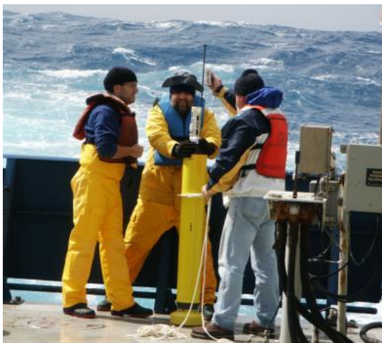
Figure 6.2 Left: Preparing an Argo profiling float for deployment (photo: A Piola). Above: Current global deployment (from http://www.argo.ucsd.edu ). Although coverage is generally good, there are still gaps associated with ice cover in the Arctic and Southern Ocean, and depth profiling is limited to ~2000 m.
